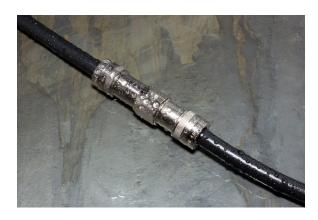
The top failure modes of coax cable assemblies in the field are caused by loose connectors or moisture entering the connector, resulting in damage to the cable and reduced system performance.
