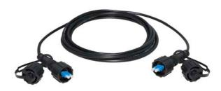
assembly is manufactured with Corning FREEDM® One cable and terminated with harsh environment connectors with strain reliefs that exceeds 56 pounds of pull. Operating temperatures are  $-40^{\circ}$  to +70 C. These harsh environment fiber optic jumpers are manufactured in New York by Cables Unlimited, a Corning Gold House.
