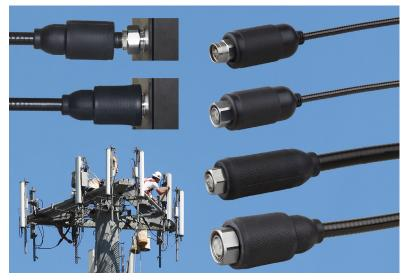
For outdoor installation of RF coaxial cable assemblies, there are numerous methods to weather-proof the connection point. Most are time consuming, expensive or difficult to install. RF Industries offers a quick and easy solution with slide on weather-proof boots. The boots come preassembled on the cable assemblies. Simply slide the boot over the mated connectors. Once the connection is fully covered, the boot provides a weather proof seal that meets IP68 rating.
