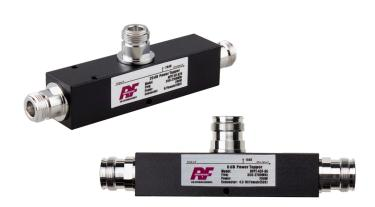
In most cases, tappers are interchangeable with couplers for Distributed Antenna System (DAS) applications. The biggest difference is a tapper does not exhibit the directionality of a coupler. Due to their lower cost, tappers have displaced couplers in many DAS installations where multiple passive devices are required.
