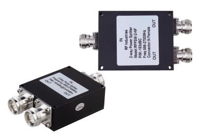
Power splitters are one of the passive components used in DAS (Distributed Antenna Systems). Also known as power dividers, splitters evenly split the RF signal to 2 or more ports that allow 2 or more antennas to be connected to a single RF signal source. Splitters are available in 2 types: reactive and resistive (Wilkinson type). Wilkinson type power splitters are more compact and offer better isolation between ports. Reactive power splitters offer a higher power rating.
