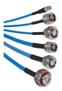
Distributed Antenna Systems (DAS) installations in buildings use large numbers of coaxial cable assemblies with special requirements. The assemblies need to efficiently transfer the RF signal (low loss), reduce the occurrence of interference caused by intermodulation (low PIM), fit into tight mechanical spaces (flexible) and meet building fire codes (plenum rated). Most coaxial cable assemblies meet some of these requirements, but fall short of meeting them all.
