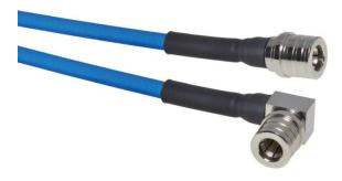
LTE networks are more acute in decreased system performance due to interference caused by Passive Intermodulation (PIM) in Distributed Antenna Systems (DAS). Traditional cable assemblies with QMA connectors may be a source of PIM. QMA connectors feature a snap lock connection as an alternative to threaded SMA connectors. QMA, with excellent electrical performance up to 6 GHz, is used in wireless infrastructure applications including DAS.
