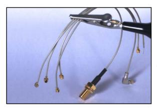
Many wireless PC board RF modules use Hirose U.FL or I-PEX MHF miniature - connectors. Jumper cables are used to connect the PC board to the device housing or case. RF Connectors, a division of RF Industries, offers the MHF series coax cable jumper. These cables use the I-PEX brand MHF connector and 1.13 mm coax cable that is compatible with Hirose U.F.L. Assemblies are available with a variety of connector terminations including SMA reverse polarity, TNC female or reverse
