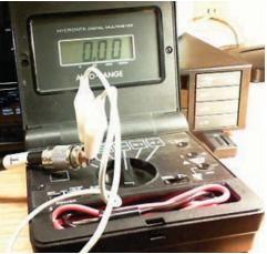
*Figure 3. Simple go/no-go continuity test for cable/connector.*
