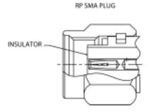
Reverse polarity SMA connectors share the same performance characteristics of standard SMA's, but the pin and socket are reversed. If you are looking into the shell of the male connector and see a flush socket and dielectric rather than raised pin, you have a reverse polarity SMA male. A raised pin in an SMA female connector indicates reverse polarity SMA female.
