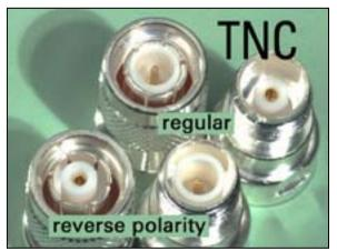
The TNC, Threaded Neill Concelman, was designed as a 7/16-28 threaded version of the 50 ohm BNC connector in the late 1950's to ensure that the connectors not de-couple during intense vibration. TNC's are weatherproofed with an internal gasket and operate from DC to 11 GHz. Internally they are identical to BNC connectors and meet MIL-39012 and MIL-STD-348. The standard TNC male has a rotating shell with gasket, slotted ground ring with dielectric material
