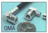
QMA connectors are quick disconnecting versions of SMA connectors; they snap on and off rather than mate by turning threads. QMA's couple in two seconds rather than twenty, but more importantly, they can be rotated 360 degrees after they are mated, optimizing the flexibility of installations and durability of jumpers. The QMA coupling mechanism creates a 360-degree butt joint that is maintained even with rotation, resulting in
