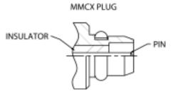
The MMCX, "miniature MCX", micro-miniature series of  $50\Omega$  connectors was developed in the 1990's for use with densely packed PCB layouts. They are about half the size of the SMB. Their lock-snap coupling mechanism with non-slotted outer contact allows 360 degree rotation without loss of broadband performance and with low
