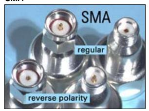
SMA, SubMiniature version A connectors (sometimes called OSM) were designed by Bendix Scintilla Corporation in the 1960's as 50  $\Omega$ , semi-precision units with small size, 1/4"-36 threaded coupling and high mechanical durability. They conform with MIL-C-39012 and CECC 22110/111 and are one of the most commonly used RF/microwave connector types used for frequencies from DC to 18 GHz. When used with miniature flexible cables their range is up to 12.4 GHz.
